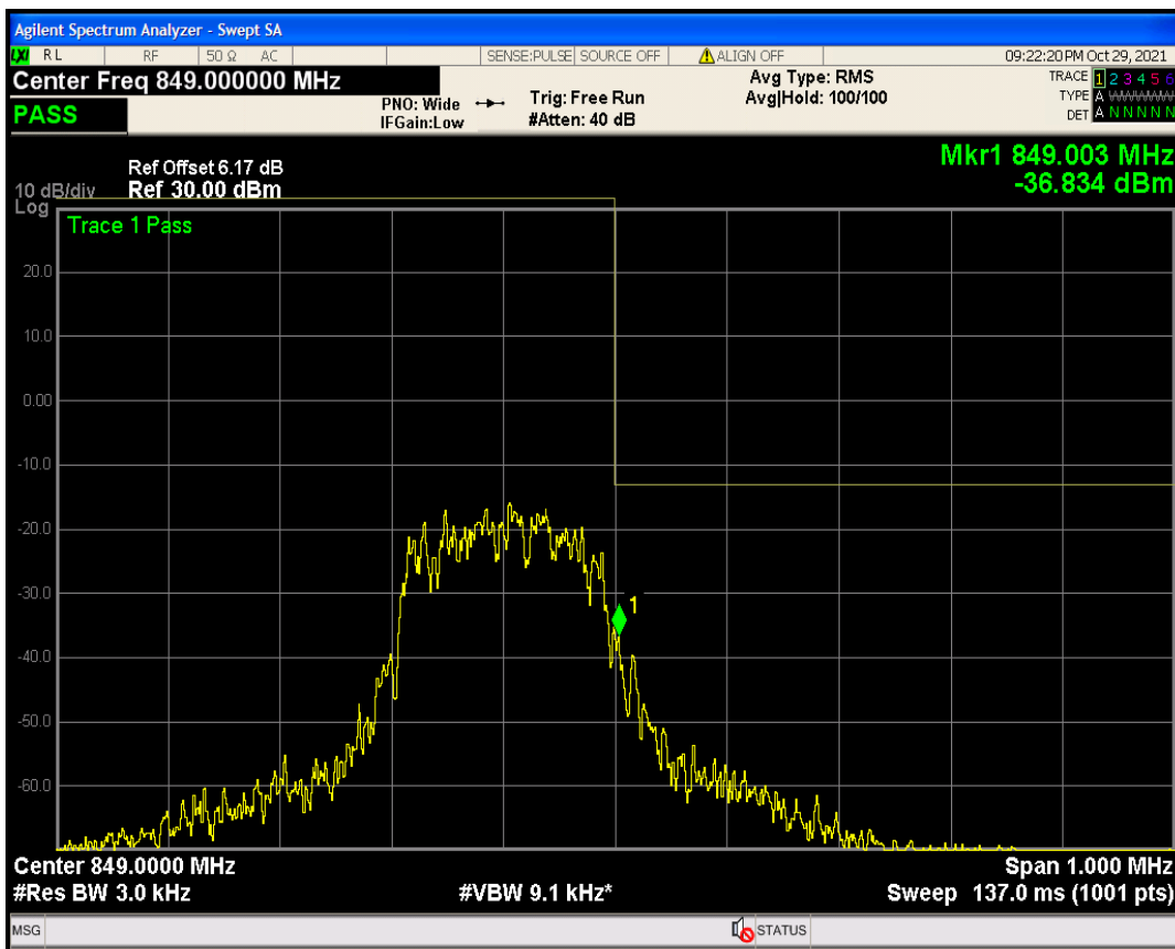
Band5 BPSK Channel=20401 nTones=1@0 Spacing=3.75kHz
