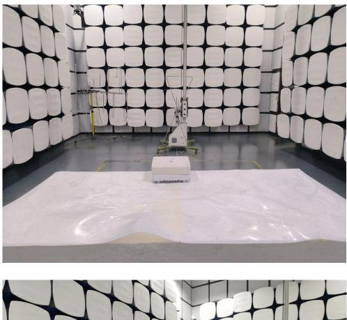
1.1. Photo of Radiated Emission test
