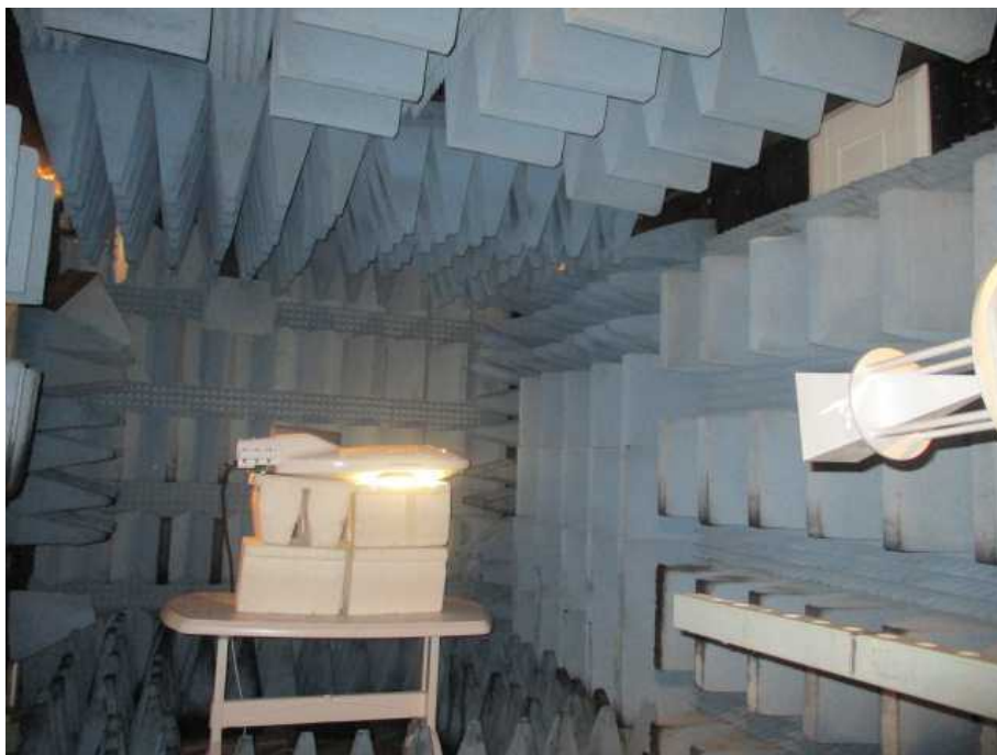
Figure 5. Radiated Emission Test, 18-26.5GHz
