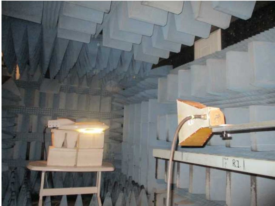
Figure 4. Radiated Emission Test, 1.0-18.0GHz
