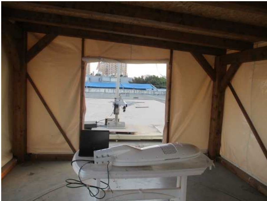
Figure 3. Radiated Emission Test, 200-1000MHz
