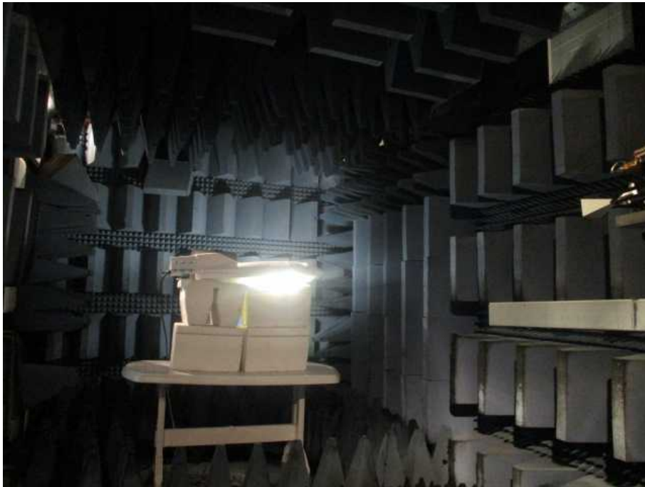
Figure 6. Radiated Emission Test, 26.5-40.0GHz
