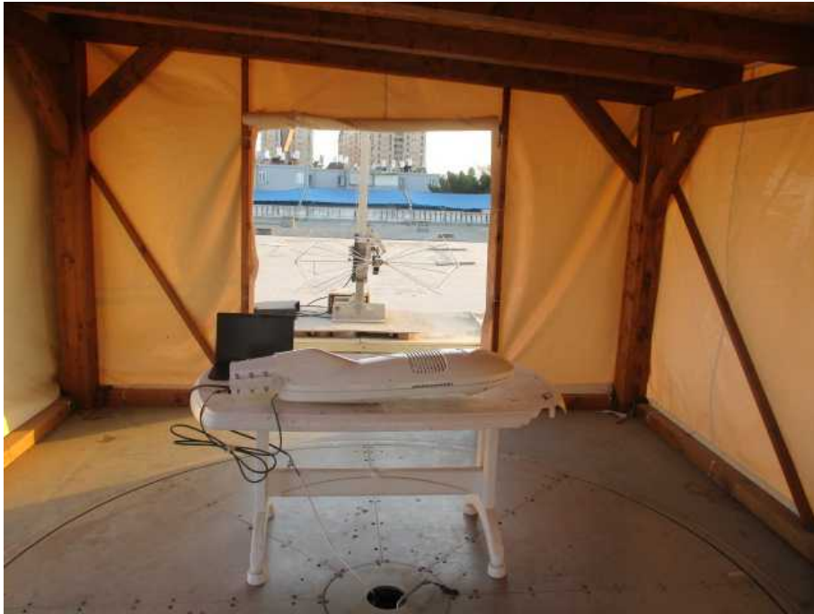
Figure 2. Radiated Emission Test, 30-200MHz
