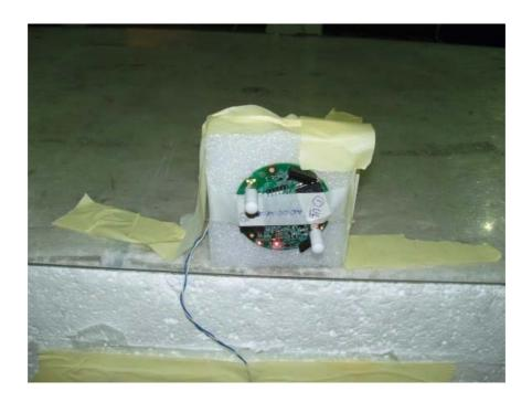
Photograph No.6 Setup for peak output power in the anechoic chamber, EUT close view in Z-axis position
