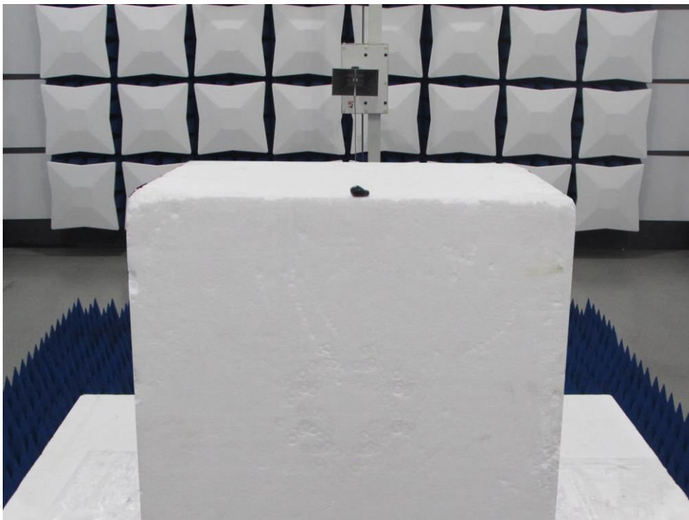
Radiated Emission Above 1GHz
