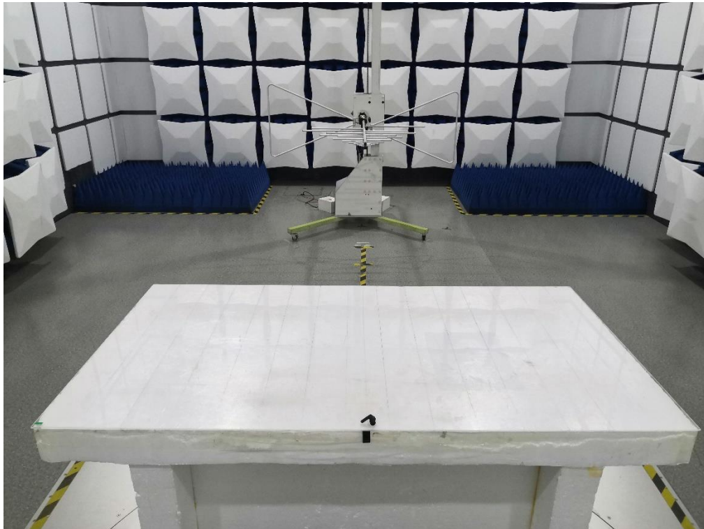
Radiated Emission Below 1GHz
