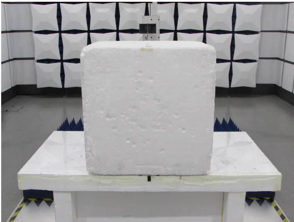
Radiated Emission Above 1GHz
