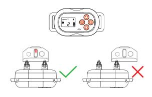
In automatic mode, the device issues a warning sound, vibration, and static stimulation the first time it exceeds the distance. Please attach the test light tool to the contact points of the device. When the static stimulation function is triggered, the test light will turn on.
