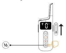
Step 2: Make sure the receiver is shut down first, and hold on the on/off button for 7 seconds. The green light will flash quickly and enter to the matching state after hearing a beep.
