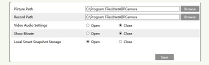
Additionally, the local smart snapshot (face snapshot) storage can be enabled/disable here.
