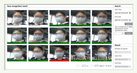
Red time tag means no comparison result. Green time tag means there is a comparison result. Click the picture with green time tag and then the face comparison information can be viewed as shown below.
