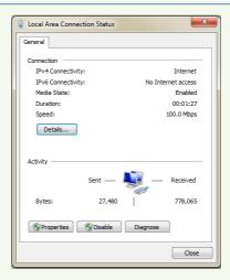
Select "Properties" and then select internet protocol according to the actual situation (for example: IPv4). Next, click the "Properties" button to set the network of the PC.
