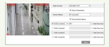
Set time stamp, device name, OSD content and picture overlap here. After enabling the corresponding display and entering the content, drag them to change their position. Then click the "Save" button to save the settings.
