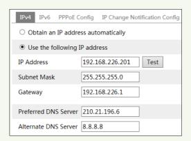
**Use IP address (take IPv4 for example)-**There are two options for IP setup: obtain an IP address automatically by DHCP and use the following IP address. Please choose one of the options as needed.
