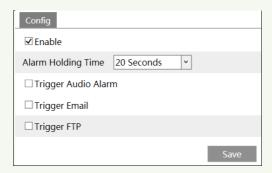
Enable "Tampering Alarm" and then set the alarm holding time and alarm trigger options.
