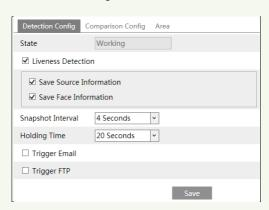
2. Enable liveness detection. If enabled, the system can distinguish real faces from non-real face spoof attacks.
