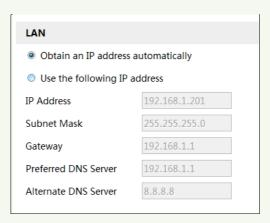
If you choose "Obtain an IP address automatically", you shall get the IP address from the router. Or you can choose "Use the following IP address" to set the network parameters manually. Then you can use this IP address to log in mobile surveillance APP/ web client/CMS/NVR/...
