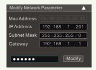
For example, the IP address of your computer is 192.168.1.4. So the IP address of the camera shall be changed to 192.168.1.X. After modification, please enter the password of the administrator and click the "Modify" button to modify the setting.
