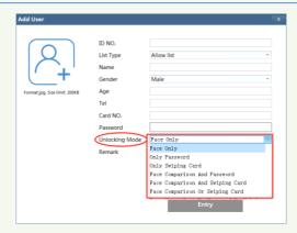
For example, supposed that the unlocking mode of someone is set to "Face Comparison and Swiping Card", this person shall be matched successfully and swipe the card on the device, and then he/she can pass.
