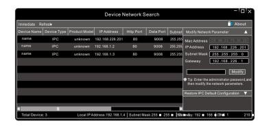
③ Double-click the camera listed in the IP-Tool or manually enter the IP address in the address bar of the web browser to connect IP camera. The default IP address of this camera is 192.168.226.201.
