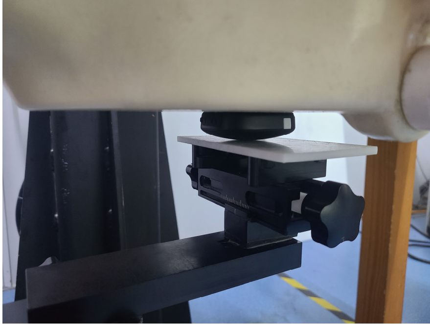
Body Back Setup Photo (0 mm)
