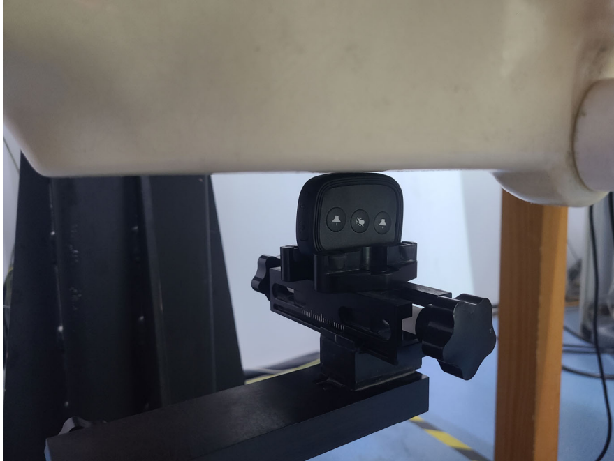
Body Right Setup Photo (0 mm)
