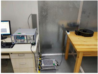
Radiated Spurious Emissions From 30MHz-1000MHz
