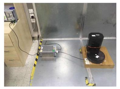
Radiated Spurious Emissions Test Frequency From 30MHz-1000MHz
