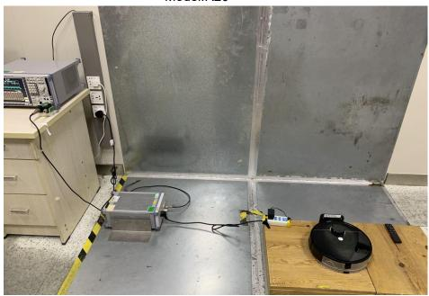
Radiated Spurious Emissions From 30MHz-1000MHz
