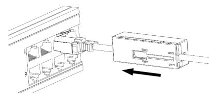
• Push the **EP-RJ45** device all the way forward towards the RJ45 port. You will hear a series of clicks as it locks on the the port.
