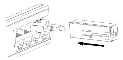
• Close the lid of the **EP-RJ45** and install the **EP-RJ45** device onto the **Unused port lock**. You will hear a series of clicks as it locks onto the port.
