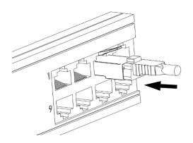
• Insert the **Unused port lock** into the RJ45 port.
