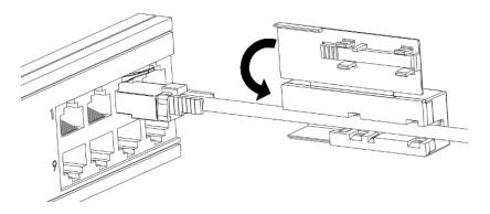
• Close the lid of the **EP-RJ45** around the in-use network cable.
