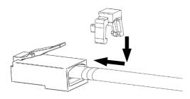
• Place the **upper cable lock** onto the network cable and into the rear of the RJ45 housing. *Depending on the style of housing, you may need to trim one or both of the tabs on the upper cable lock.*
