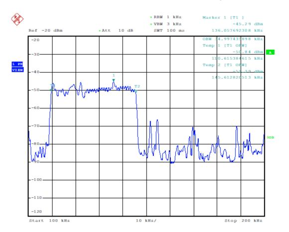
According the test data above, the fundamental wave is not fall in the restricted band 90KHz-110KHz, the field strength also meet the 15.209 requirement, so this test is Pass.
