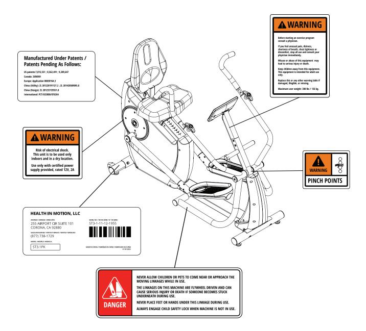
THE WARNING AND PATENT LABELS HAVE BEEN PLACED ON THE UNIT IN LOCATION SHOWN. IF THE LABELS ARE MISSING OR ILLEGIBLE, PLEASE CALL CUSTOMER SERVICE AT +1 877-738-1729 FOR REPLACEMENTS. APPLY THE LABELS IN LOCATION SHOWN.
