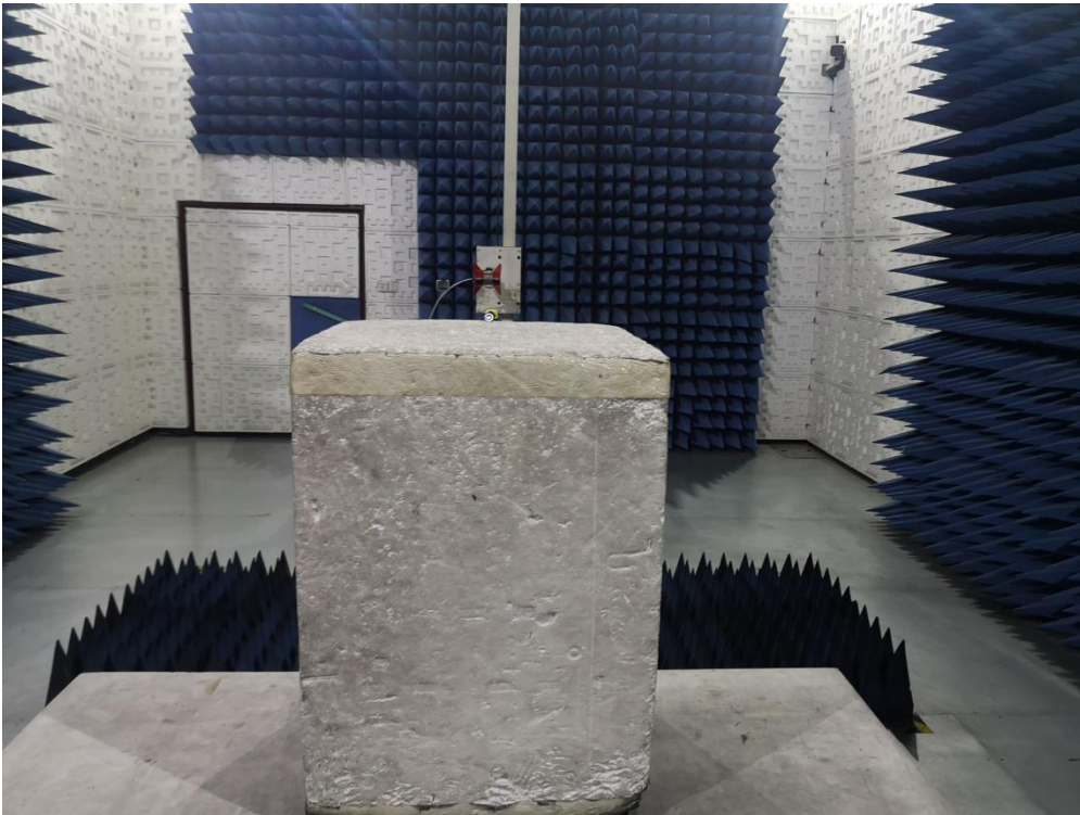
RADIATED EMISSION TEST SETUP ABOVE 1GHz
