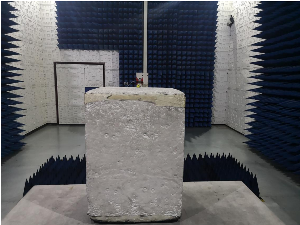
RADIATED EMISSION TEST SETUP ABOVE 1GHz
