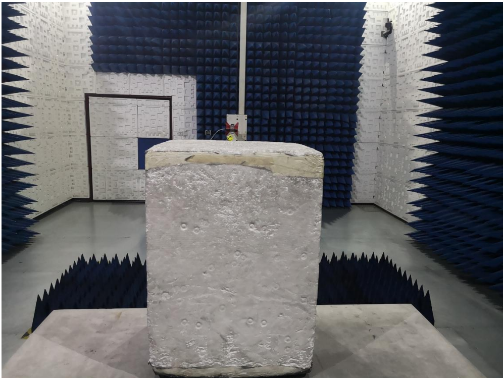
RADIATED EMISSION TEST SETUP ABOVE 1GHz
