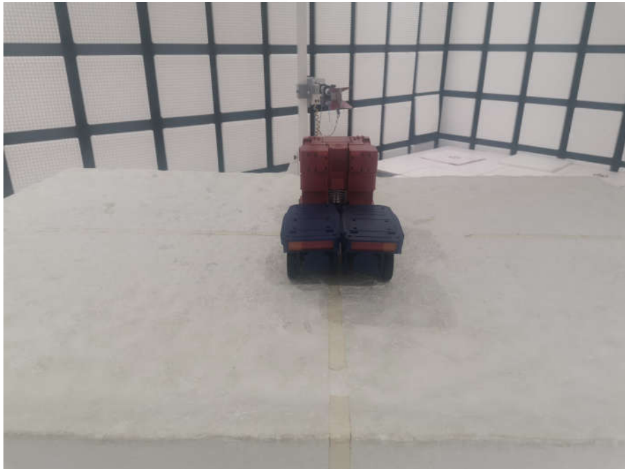
Radiated spurious emission Test Setup-2(Above 1GHz)
