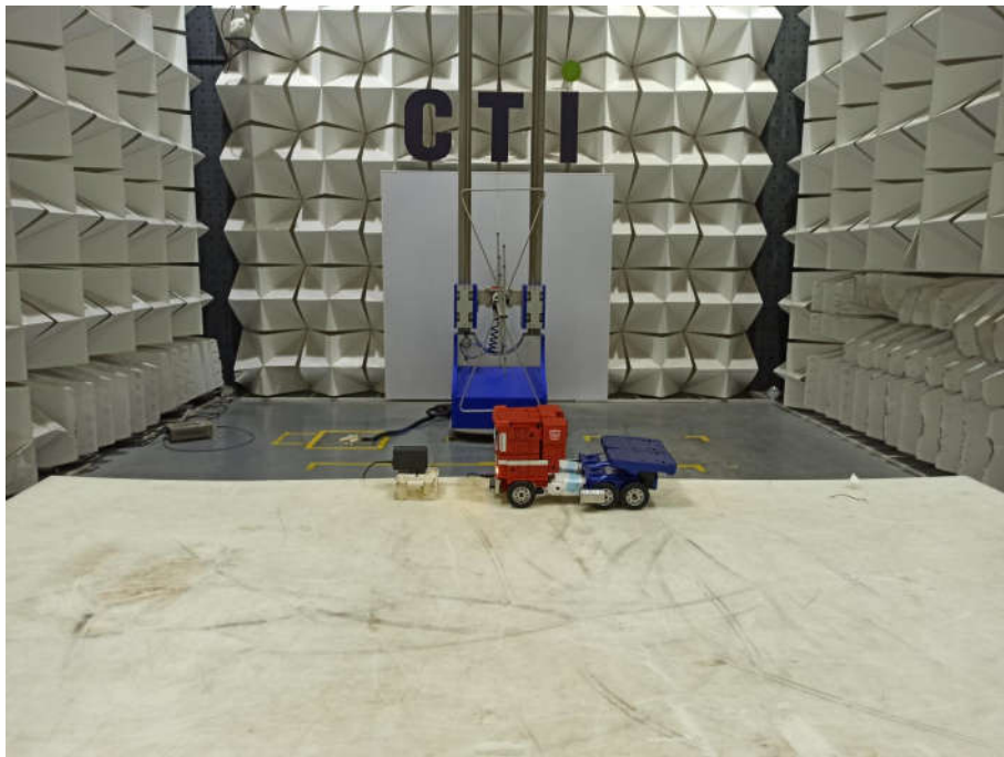
Radiated spurious emission Test Setup-2(Below 1GHz)
