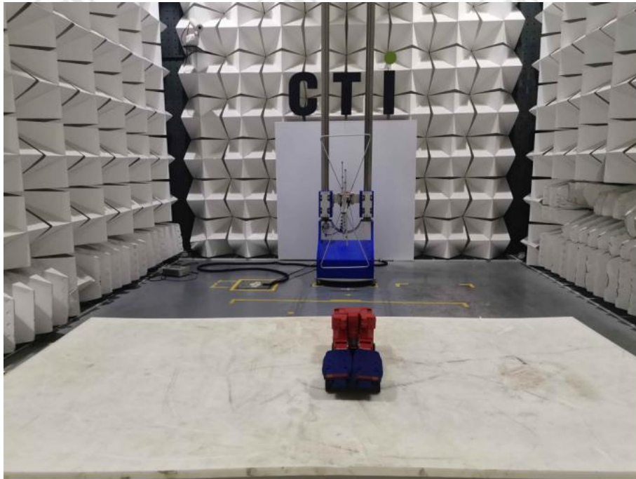
Radiated spurious emission Test Setup-1(Below 1GHz)
