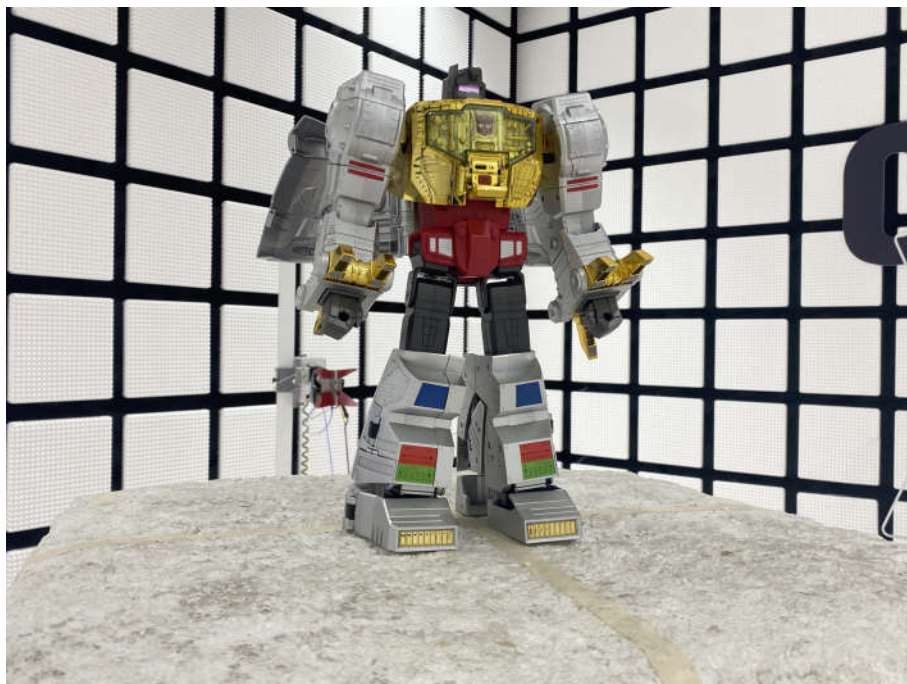
Radiated spurious emission Test Setup-2 (Above 1GHz)
