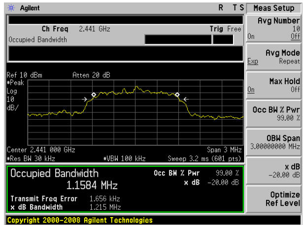
20dB Bandwidth plot on channel 78 (2Mbps)
