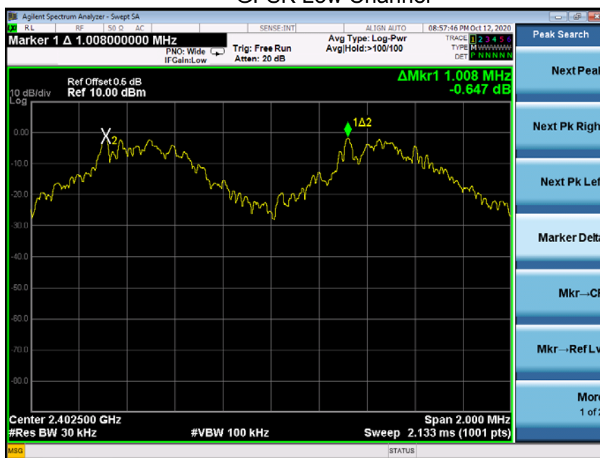
Test plots GFSK Low Channel
