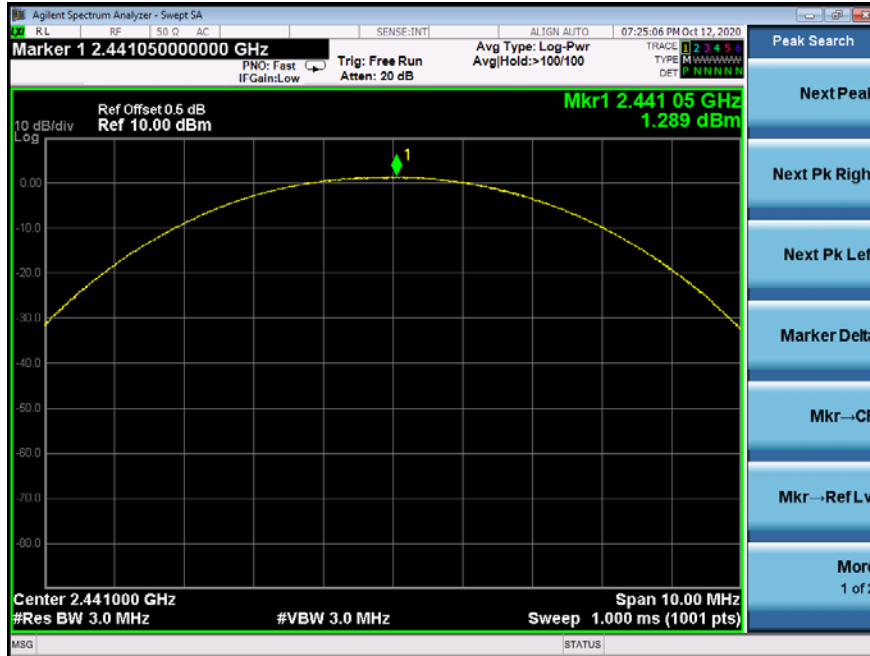
Pi/4 DQPSK Middle Channel
