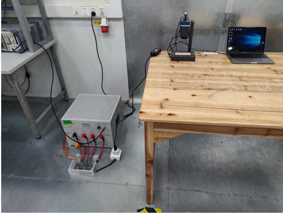
Photo of Conducted Emission Measurement
