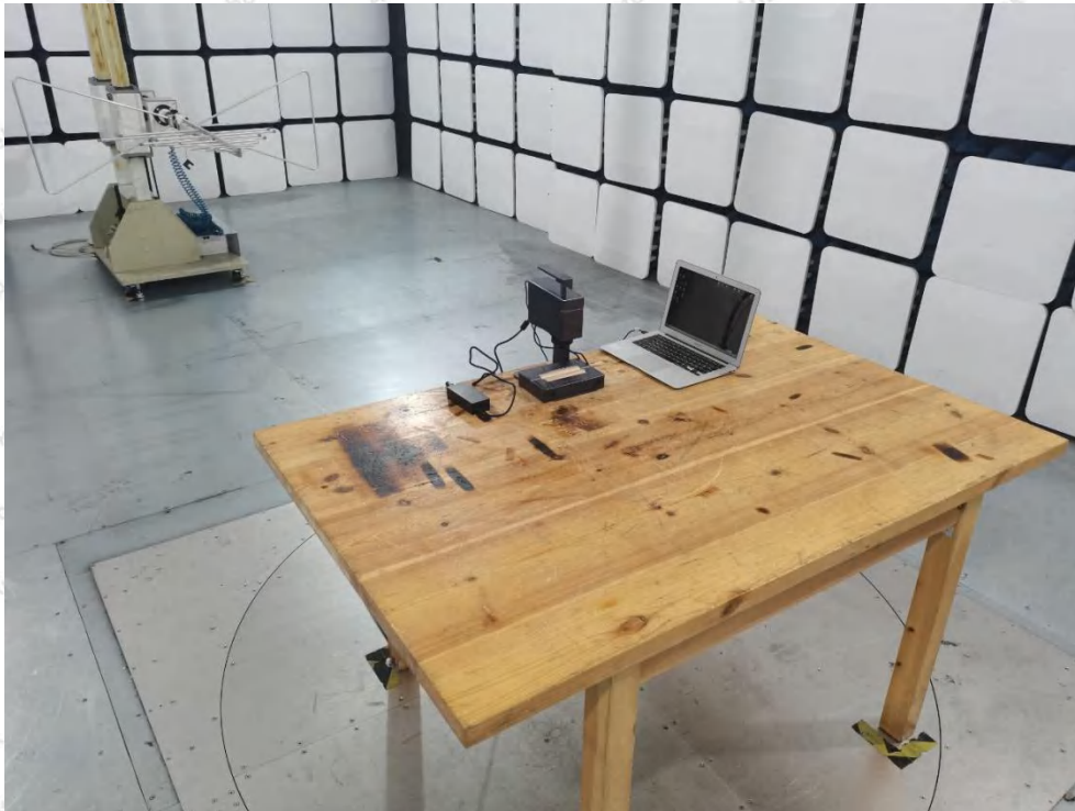
Photo of Radiation Emission Test
