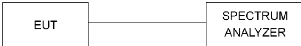
Figure 1 – Conducted Measurement Test Setup
