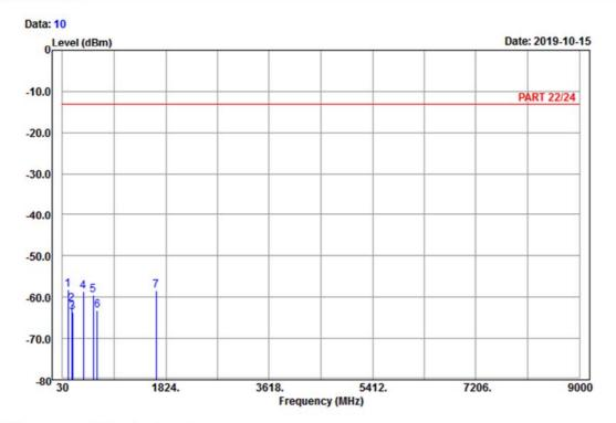
Site : 966 chamber 1 Condition: PART 22/24 Vertical Remark : Band V\_Link\_L-Ch Tested by: Charles Hsiao
