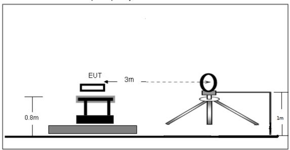
(B) Radiated Emission Test-Up Frequency 30MHz~1GHz
