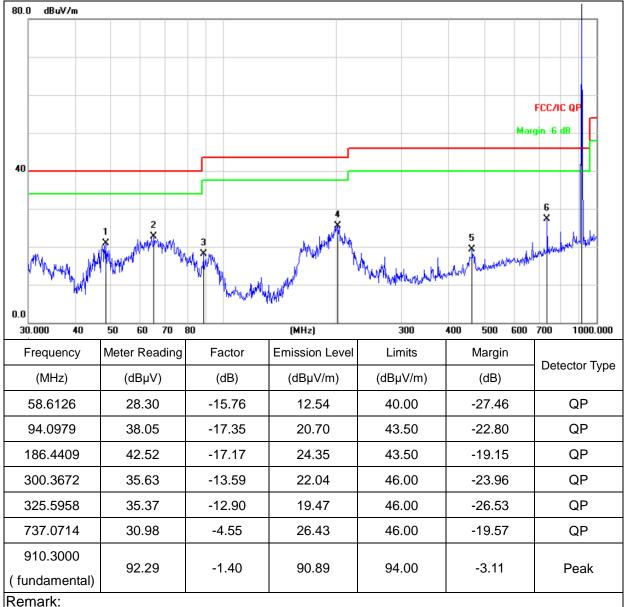
Factor = Antenna Factor + Cable Loss – Pre-amplifier.
