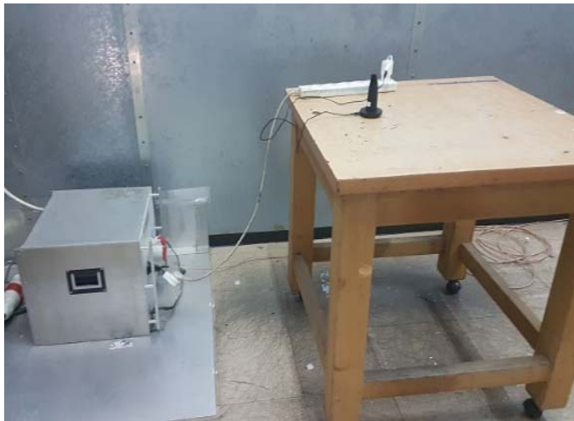
Photo 6. Conducted emissions test setup (Charging)
