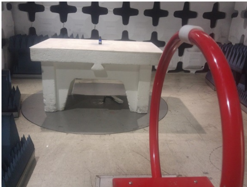
Photo 1. Radiated emissions test setup with Loop antenna.
