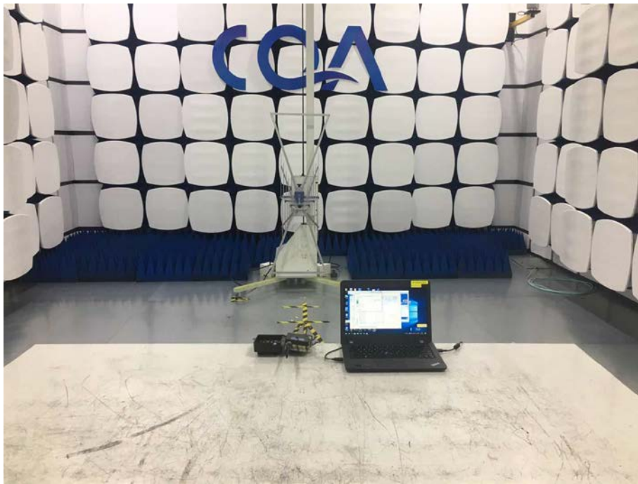
Radiated emission Test Setup-2 (30MHz~1GHz)
