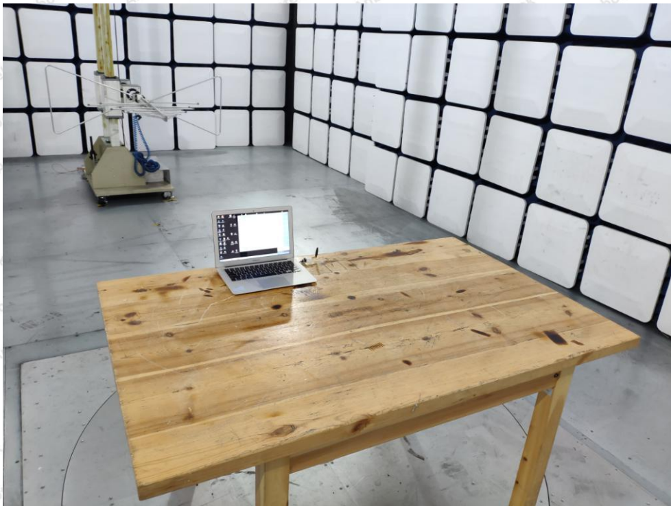
Photo of Radiation Emission Test
