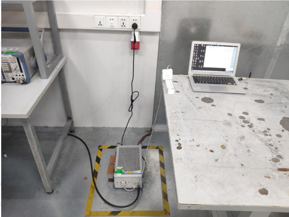
Photo of Radiation Emission Test
