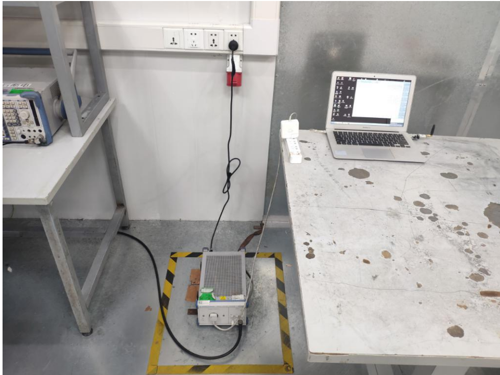
Photo of Radiation Emission Test
