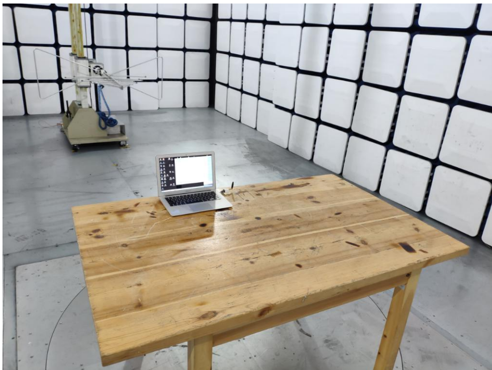
Photo of Radiation Emission Test
