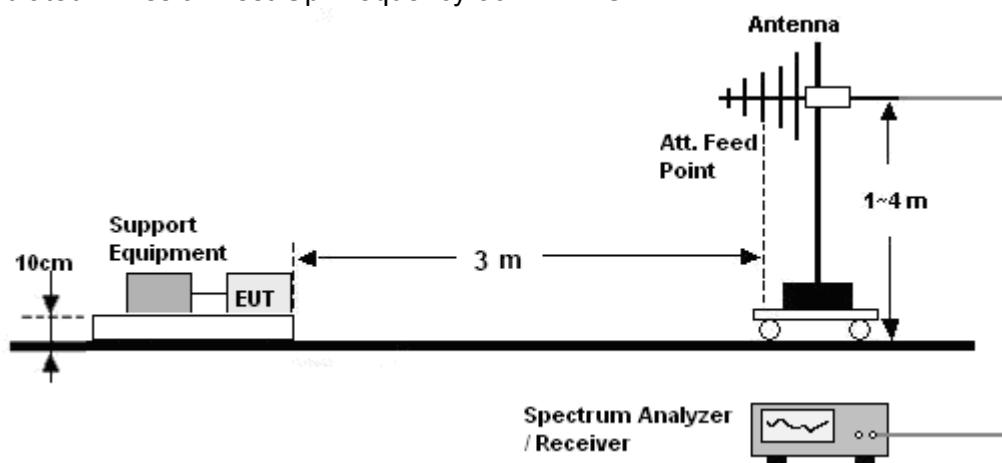
(C) Radiated Emission Test-Up Frequency Above 1GHz
