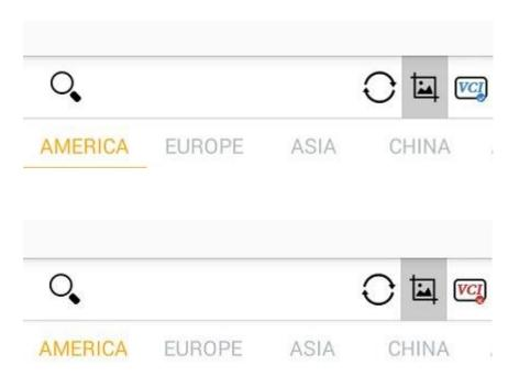
3. If the M400 cannot automatically connect to your VCI device, or the device fails to connect, please manually click the VCI icon on the top right to reconnect, or check whether the VCI is well connected to the car's OBD port.
