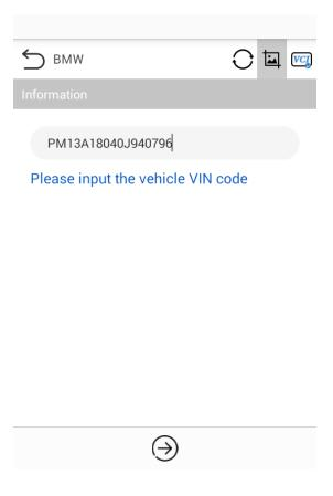
After the vehicle information is selected. Tap the NEXT button at the bottom right corner of the screen to open the Main menu page. This section consists of various functions commonly used, including quick test, system selection, and more. The available functions displayed vary by vehicle.
