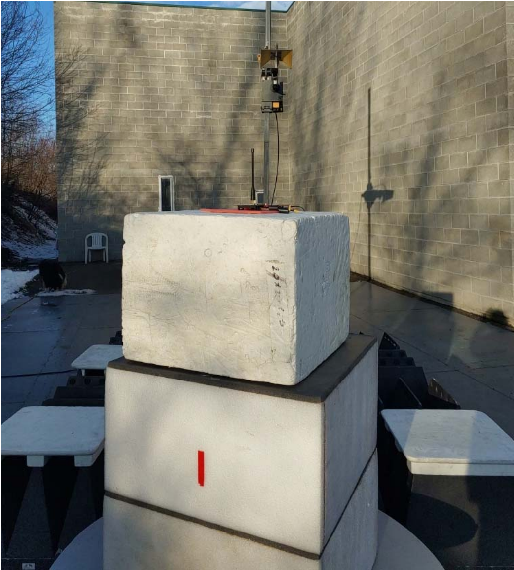
Figure E21.5 – Test Set Up - Radiated Measurements 1 – 4GHz, Antenna #1
