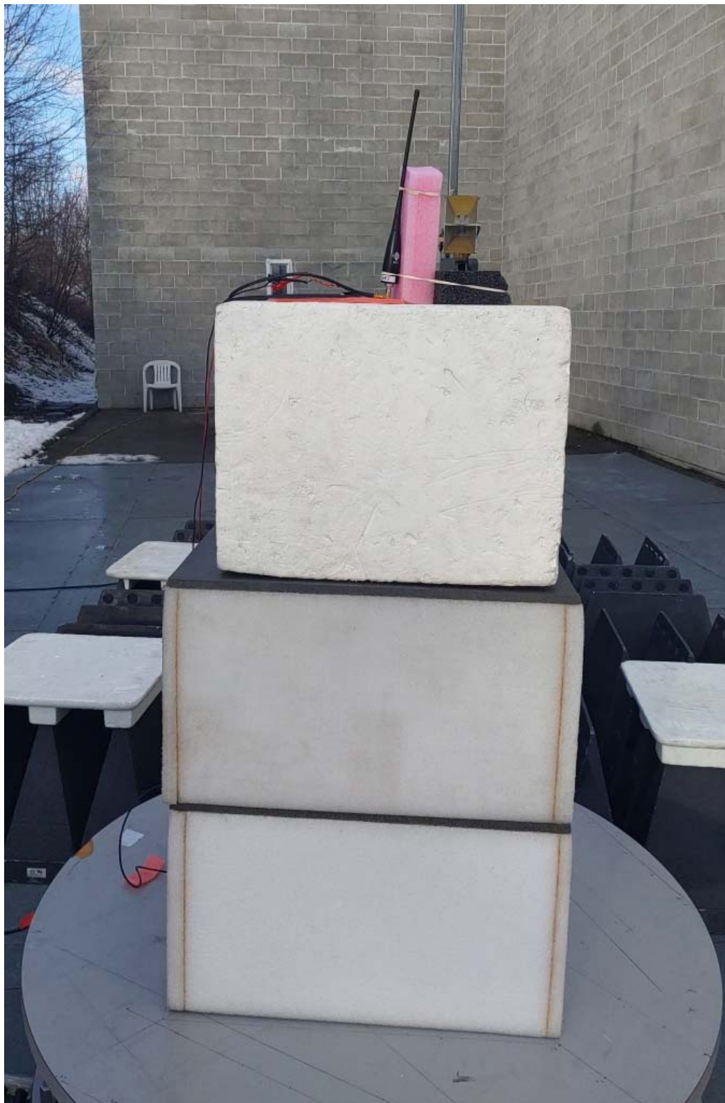
Figure E21.6 – Test Set Up - Radiated Measurements 1 – 4GHz, Antenna #2
