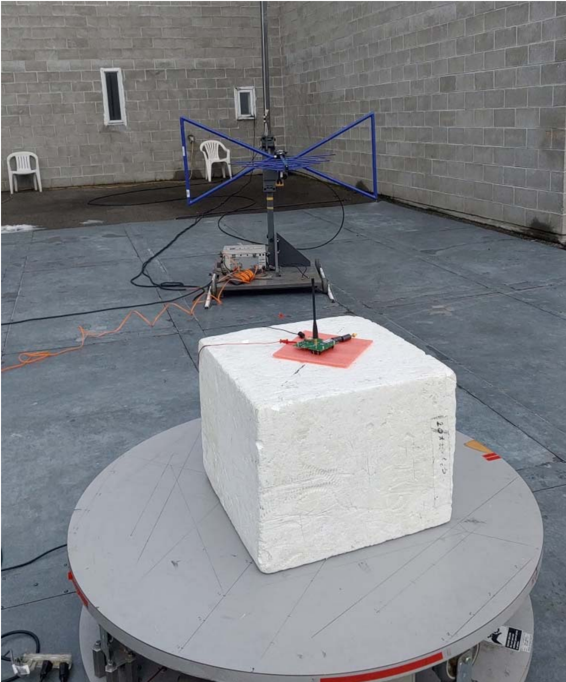
Figure E21.3 – Test Set Up - Radiated Measurements 30MHz – 1000MHz, Antenna #1
