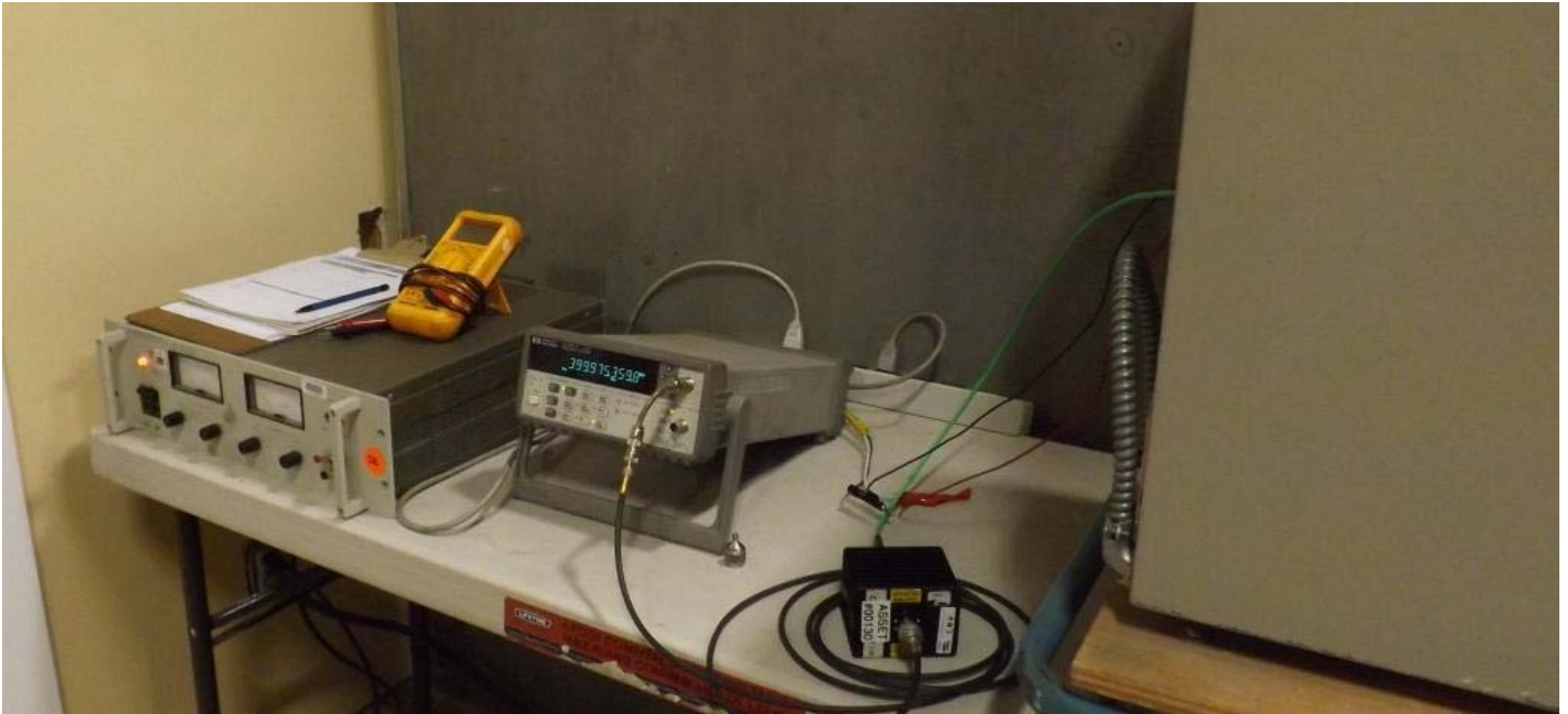
Figure E21.7 – Test Set Up - Frequency Stability
