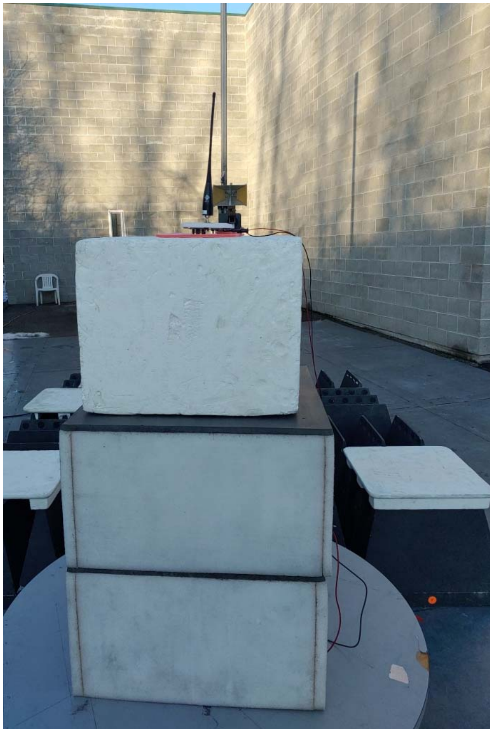
Figure E21.4 – Setup Photo – Radiated Rx, 1 – 5GHz, Antenna B
