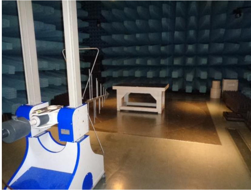
Figure 9.1-1: Radiated emissions set-up for frequencies below 1 GHz
