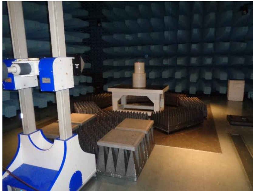
Figure 9.1-2: Radiated emissions set-up for frequencies above 1 GHz
