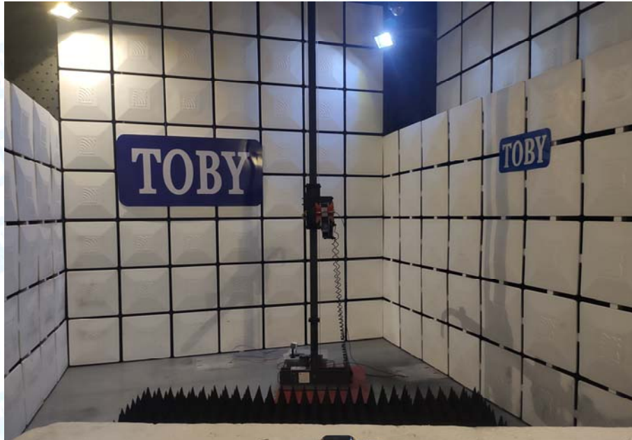
Photo of Setup for Radiated Emission (Above 1 GHz)
