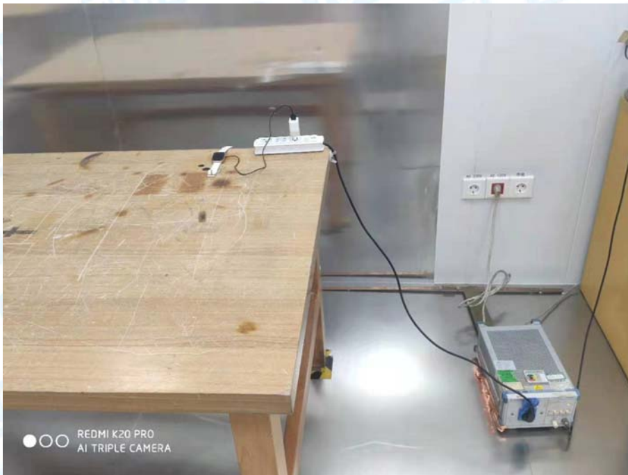
Photo of Setup for Conducted Emission
