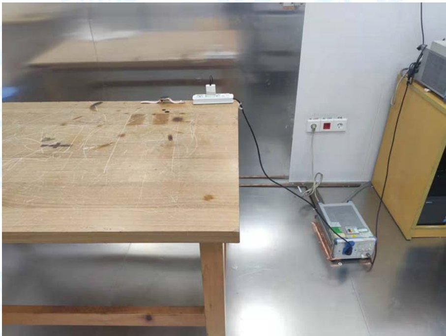
Photo of Setup for Conducted Emission
