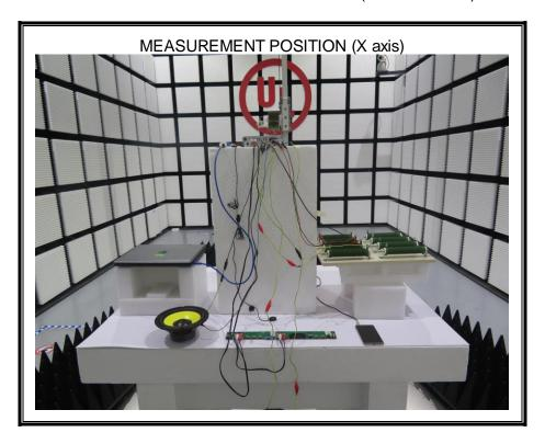
RADIATED RF MEASUREMENT SETUP (30MHz~1GHz)
