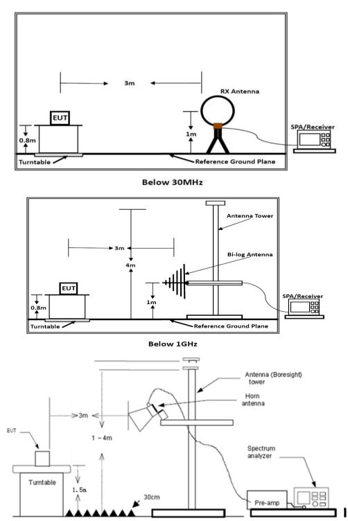
Above 18 GHz shall be extrapolated to the specified distance using an extrapolation factor of 20 dB/decade form 3m to 1m.
