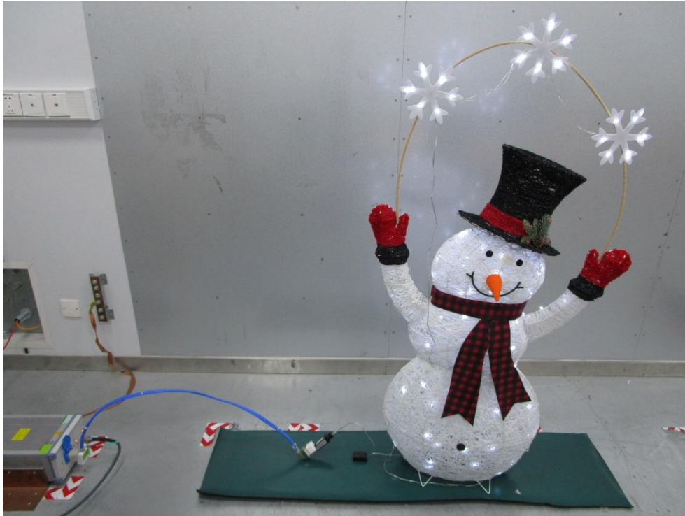
Conducted Disturbance test setup photo
