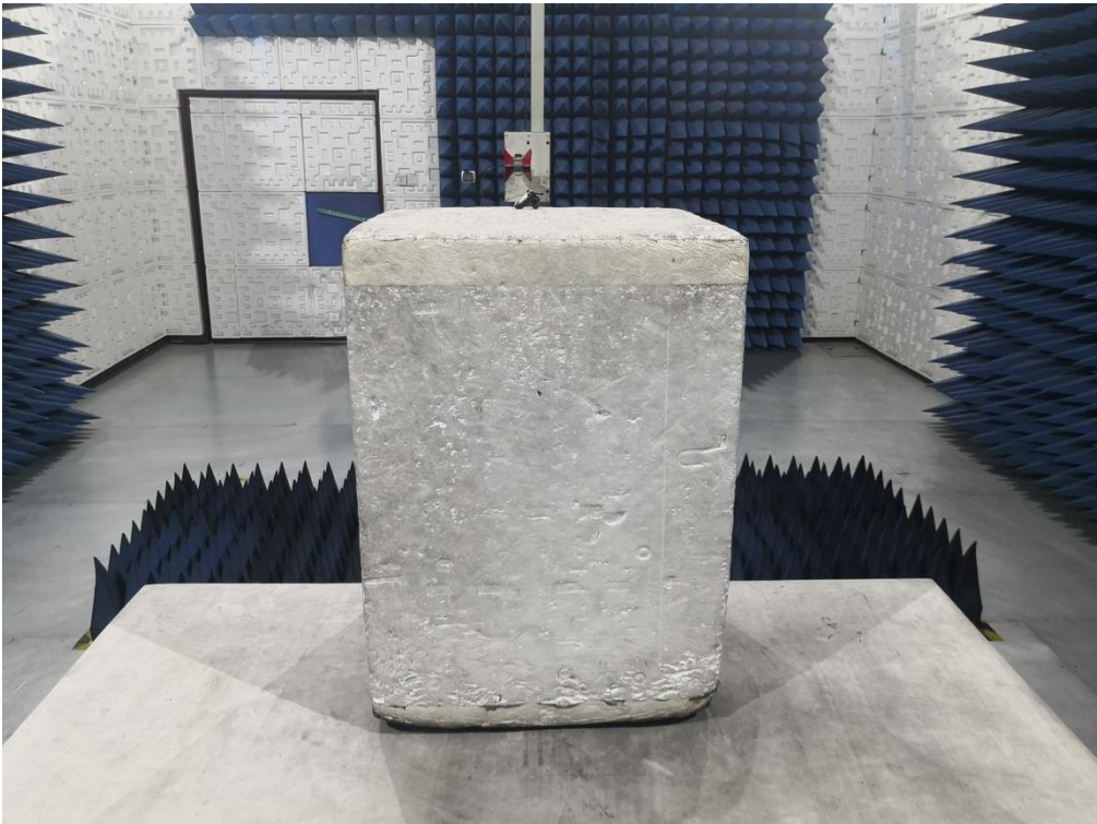
RADIATED EMISSION TEST SETUP ABOVE 1GHz
