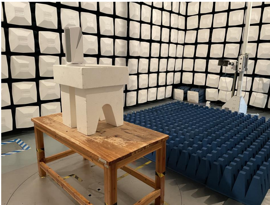
Test Setup For Radiated Emission (Above 1GHz)
