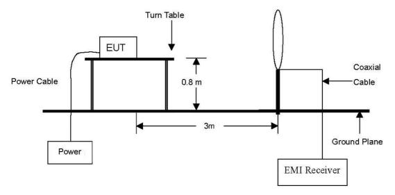
The diagram below shows the test setup that is utilized to make the measurements for emission from 30 Mz to 1 GHz.
