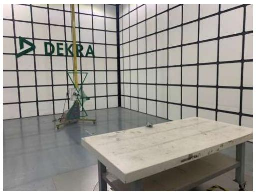
Description: Radiated Emission Test Setup for 1~18GHz
